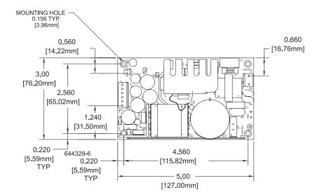
MAX. COMPONENT HEIGHT1.20" [30.28 mm] MAX. LEAD PROTRUSION 0.10" [2.54mm]
